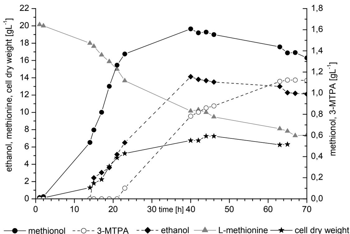
**Figure 2.** Bioprocess kinetics of the production of methionol with *S. cerevisiae* CEN.PK113-7D during batch cultivation in a 0.45 L bioreactor with 0.2 L working volume. Glucose was fed at a constant flow rate between  $t = 26$  h and 36 h. Reprint with kind permission of Springer [9].
