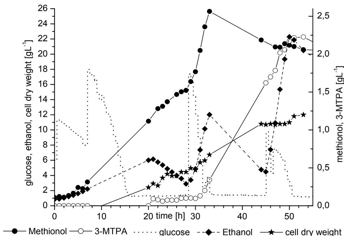
**Figure 3.** Bioprocess kinetics of *S. cerevisiae* CEN.PK834-1C in a bioreactor. Glucose was fed manually at  $t = 8$  h, 29 h, and 45 h. The glucose concentration in the reactor was monitored online. Reprint with kind permission of Springer [9].
