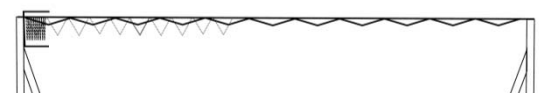
Fig. 5 New light weight PV mounting solution (A. Büchel, F. Baumgartner). In case of strong wind and snow the PV cells are parked in the safe position inside the housing on the left part of the system.
