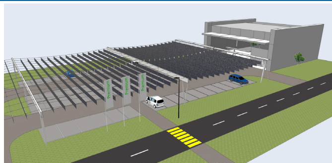
Fig. 1b LE Urban Plant Pergola –the PV modules are installed in a vertical position. Modules have an electrically active front and rear side and will not be moved into the safety box.
