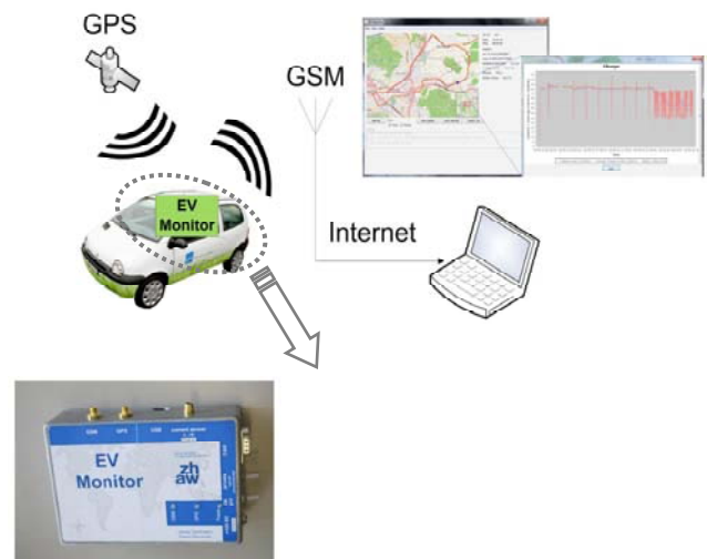
Figure 1: Overview of the concept showing the central part (EV-Monitor box built into automobile), connection to external networks and graphic interface.
