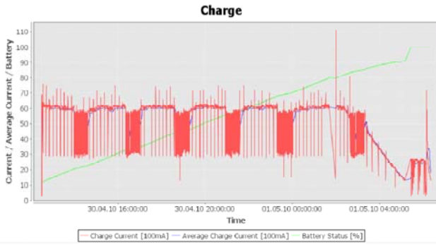
Figure 4: Measurement of a complete loading cycle with instantaneous and average (over last 50 values) current plus associated battery status (charging from 12% to 91% over 16 hours).
