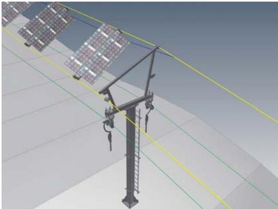
**Figure 8:** Solar Wings one-axis 60kW Ski-lift will be installed at the end of 2011 in the skiing area of Safiental, Switzerland.[5]
