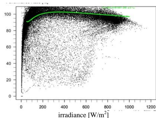
**Figure 6:** Measured Performance Ratio of the PV plant during the whole year 2009 with an average value of 92.5 for the 654.3kW nominal power[4]
