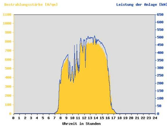
**Figure 3:** Webshot from the public ISE Sunways online monitoring portal showing the solar irradiance characteristics in the tracked module plane (left axis  $W/m^2$ ) together with the AC power feed into the grid (right axis kW) at the 19<sup>th</sup> of Oct 2009.[4]
