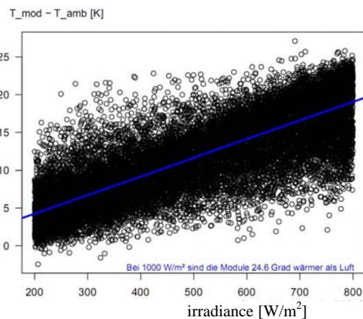
**Figure 4:** Measured temperature difference between PV modules and ambient temperature versus irradiance [ $W/m^2$ ] during 2009 (average module temperature during day time was  $25.1^\circ C$  and average ambient temp  $11.2^\circ C$  [4])
