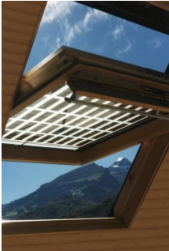
Fig. 2a First SOLAR ROOF WINDOW prototype at the outdoor test on the roof of the NTB - building. The 36Wp PV-generator consists of 66 silicon half cells (each 36x 100mm 2 ) and connected to the grid by an module - converter. (Daylight transparency of 51 percent)
