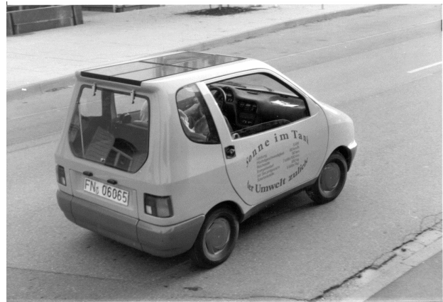
Figure 3: Solar filling station at the university building in Constance (500 Wp a-Si modules) and solar car TINO (80 Wp . roof integrated cryst. Si PV-modules)
