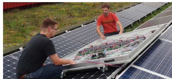
Figure 1: LED flasher in operation on a PV power plant, cover profile on the top was removed to show the power electronics on the opposite side of the LEDs
