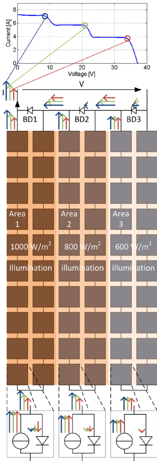
Figure 4: Bypass diode test with a 60 cell crystalline silicon module with 3 correct working bypass diodes. There are different illumination values in the 3 different sub-module areas (see Table II). The length of the arrows indicates the magnitude of current for the applied load according to the I-V scan
