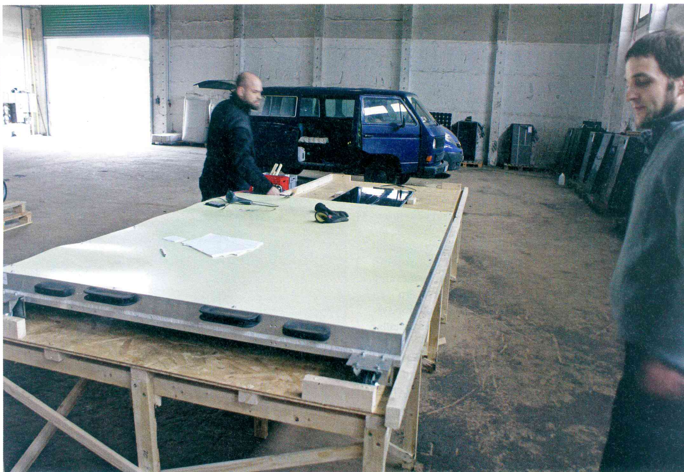
At the farm in Quedlinburg, Schär and a small team from PI Berlin work fastidiously in testing the solar panels, delivering a series of flashes designed to assess nominal power, bypass diodes and low-light performance.
